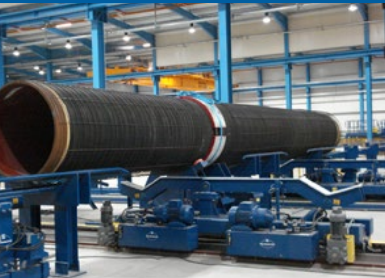
Anode on pipe
