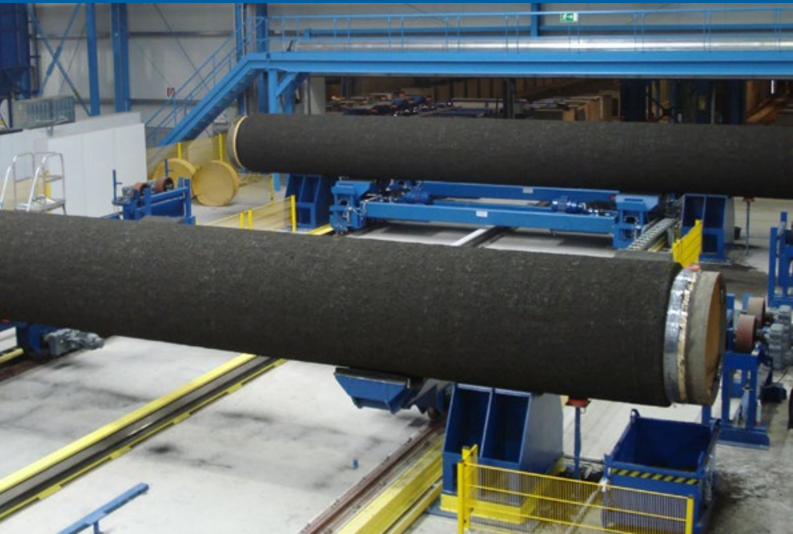
Pipe end cleaning area before curing
