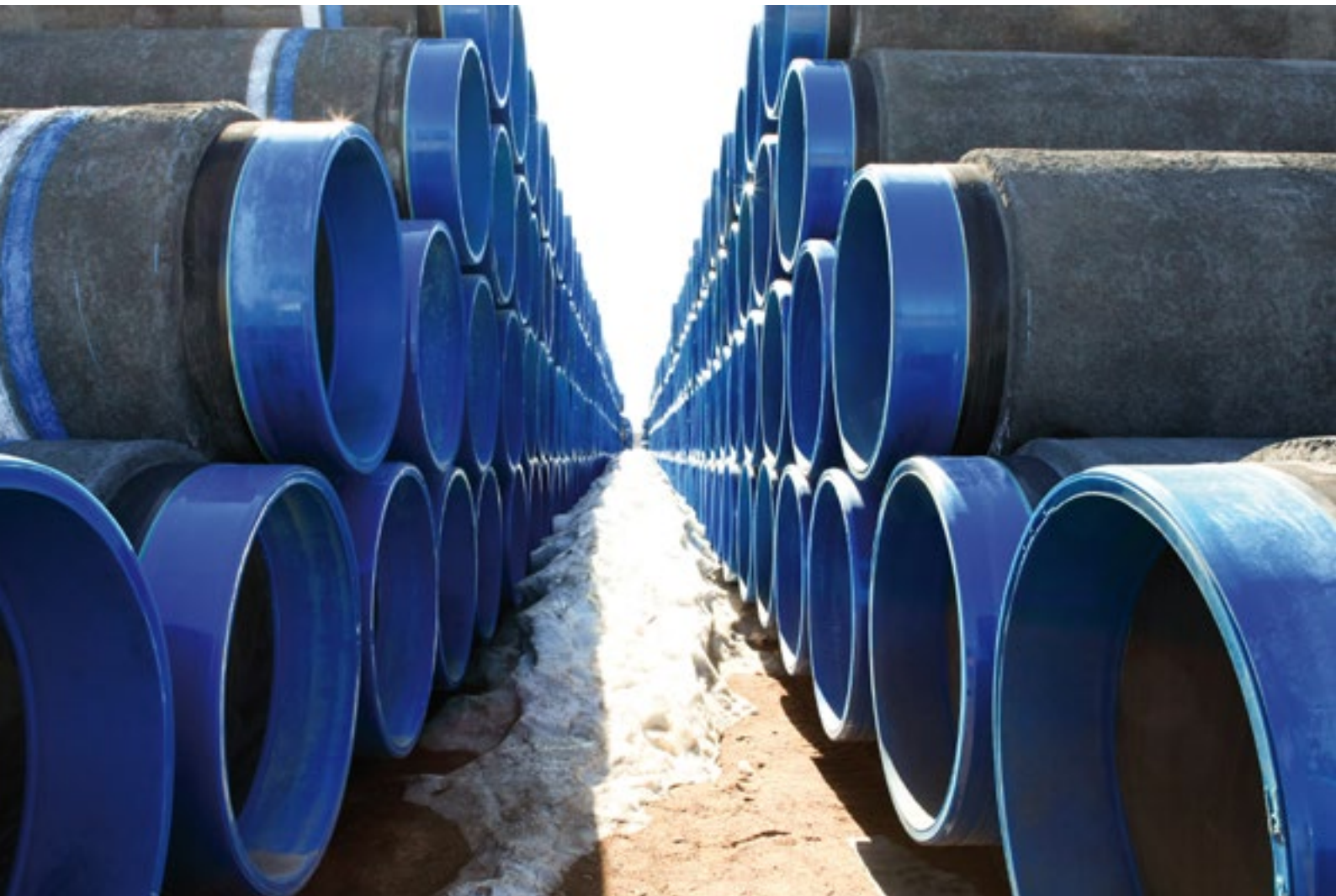
Concrete coated pipes
