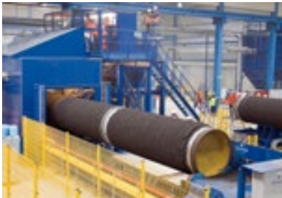
Concrete weight coating
