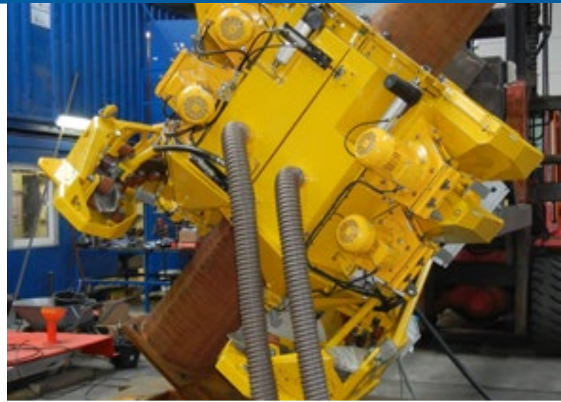
J-lay wheel blaster
