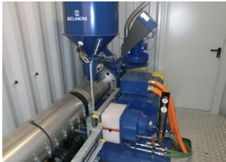
Extruder for IMPP connected to accumulator
