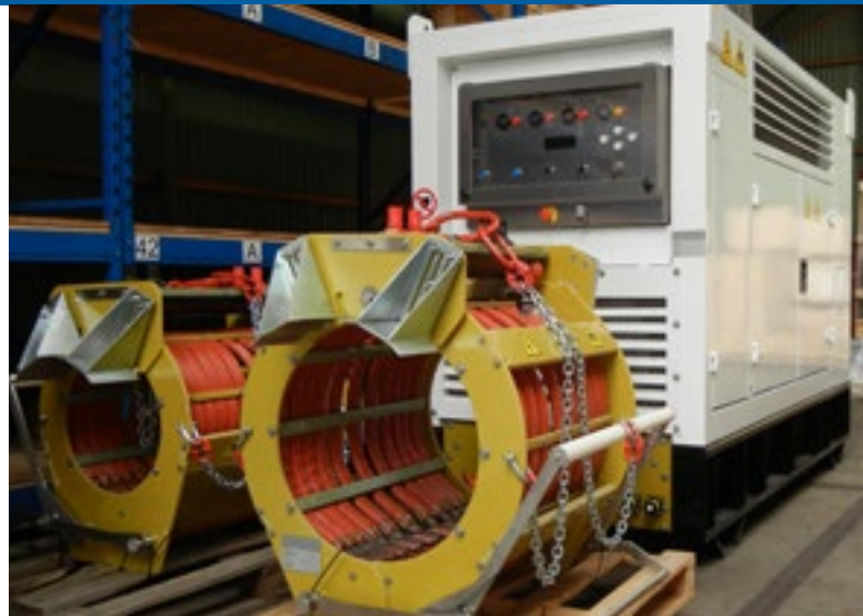
Induction heating equipment
