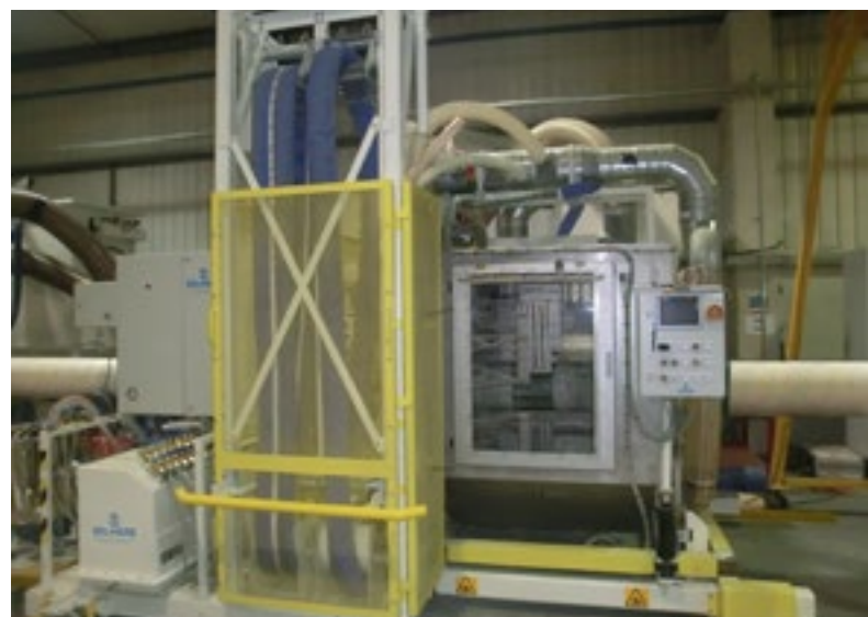
Enclosed spoolbase FBE/CMPP coater
