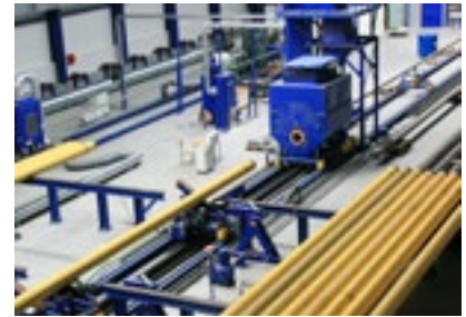
Internal blasting & lining
