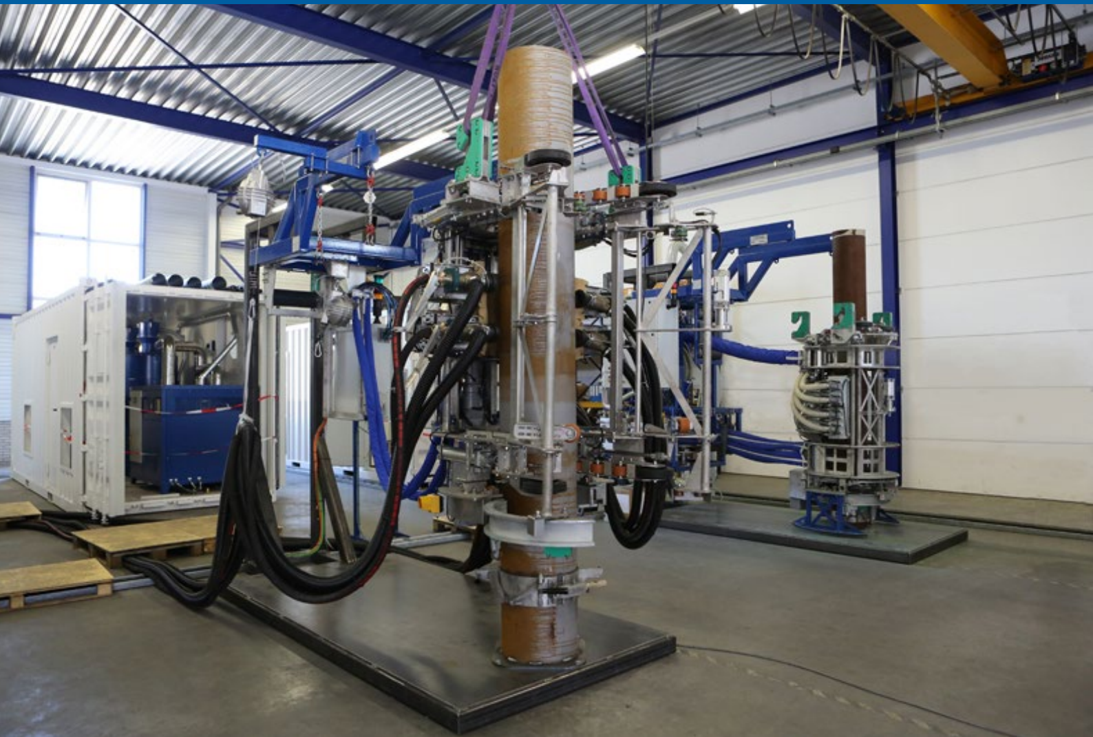
Testing of J-lay blasting and coating equipment at Selmers facility
