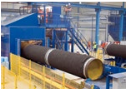
Concrete weight coating
