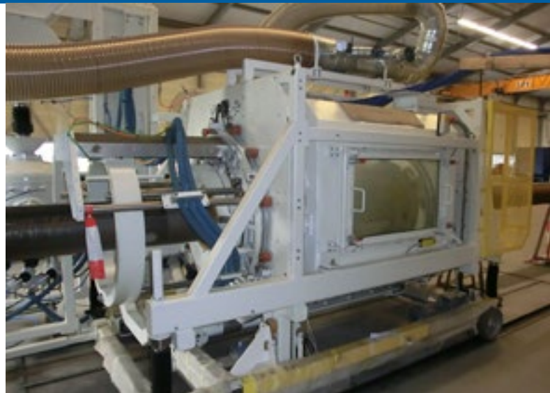
Field joint blaster in spoolbase
