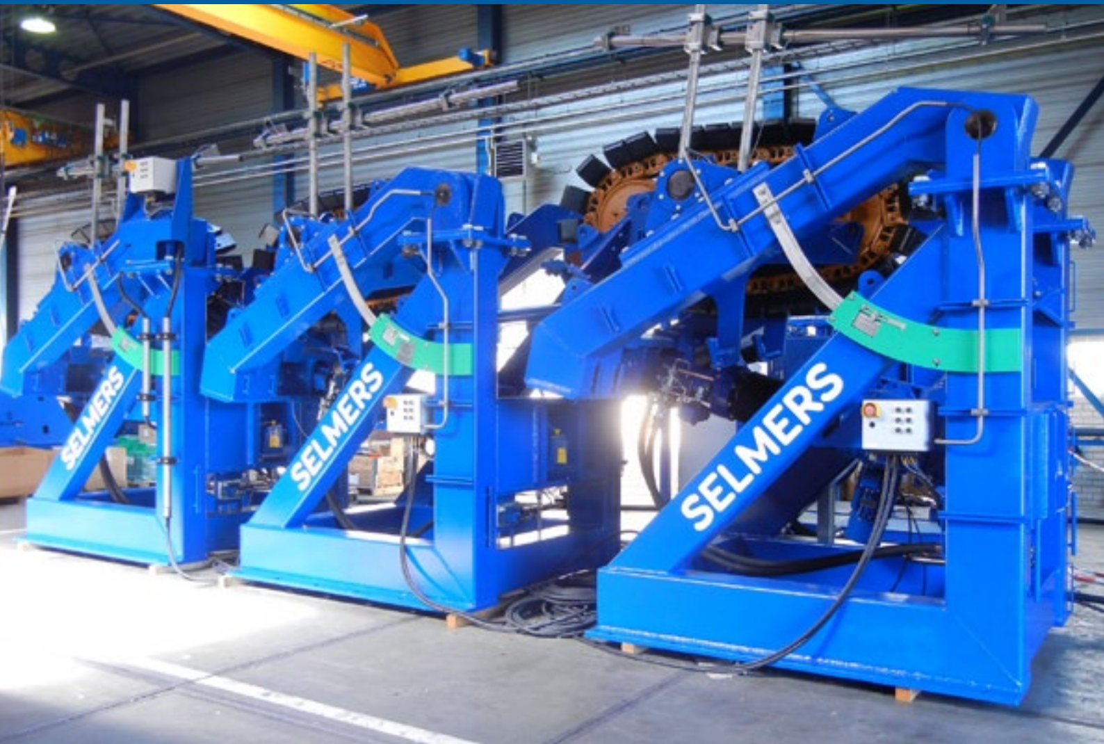
Pipe loading reaction rollers
