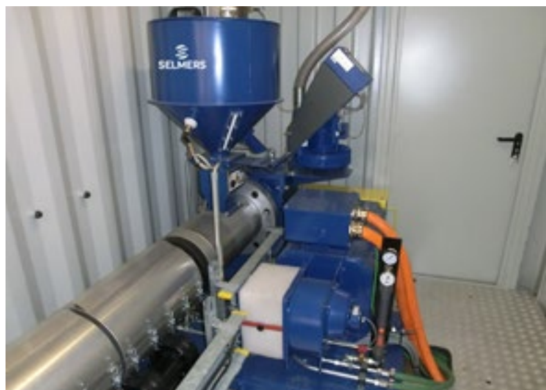
Extruder for IMPP connected to accumulator
